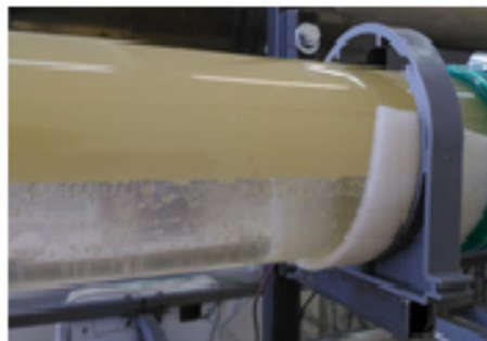
Fig. 5. The nature of the water-oil contact along the length of the horizontal pipeline
